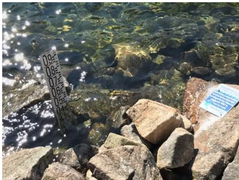
Figure 7. LOCSS ( Lake Observations by Citizens Scientists and Satellites ) and OECS ( Observations des Eaux continentales par des Citoyens et des Satellites ) in-situ rules for citizen contributions: lakes and rivers levels are sent to the project by the citizens.
