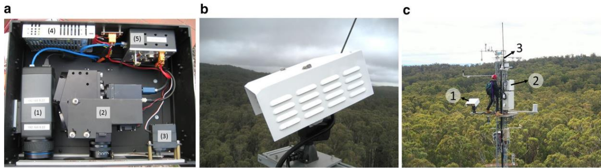
Figure 9: An internal view of the main sensor enclosure. (1) thermal camera, (2) VNIR hyperspectral line scanner with cooling fan, (3) shutter motor and mechanism, (4) 24 VDC to 12 VDC converter, and (5) shutter controller with temperature sensor. b External view of the main sensor enclosure on the pan-tilt unit tilted downward at the canopy. The white cover is a radiation shield with ventilation. c Contextual view of the THEMS sensor enclosure (number '1' insert). Other inserted numbers are 2) the command PC enclosure and 3) the all-sky camera and irradiance sensor location. (Extract from Woodgate et al. 2020).
