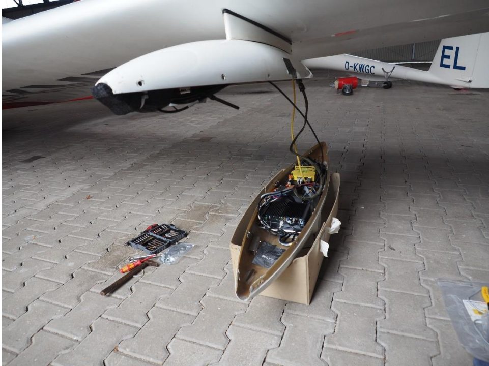
Figure 21: Wingpod version of SWING, integrated on a motor glider ASK 16 from Free University of Berlin (FUB)
