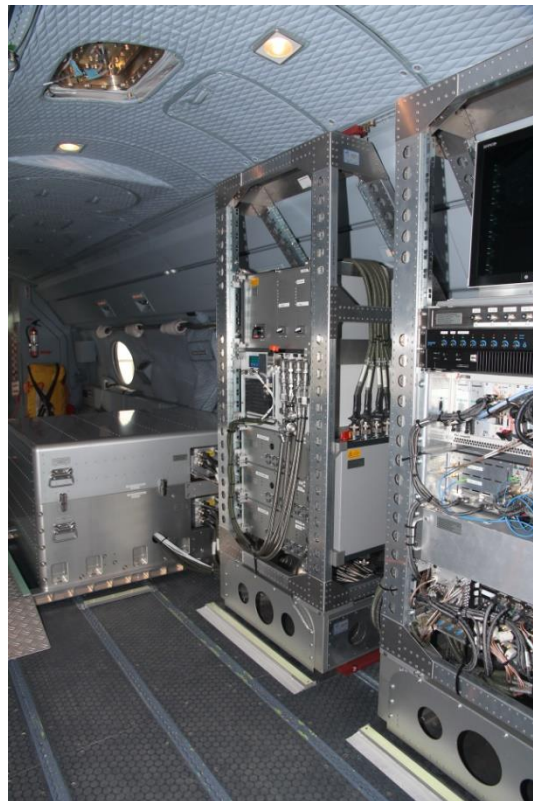
Figure 19: CHARM-F installed inside the German research aircraft HALO.
