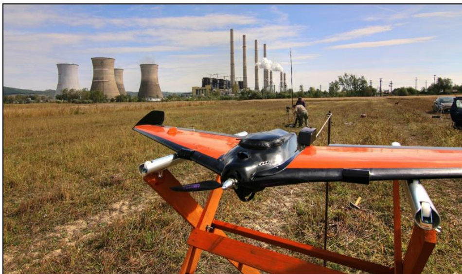
Figure 23: Example of a fixed wing UAV developed by Reev River Aerospace and operated with the BIRA SWING instrument during the AROMAPEX campaign (Merlaud et al., 2018).
